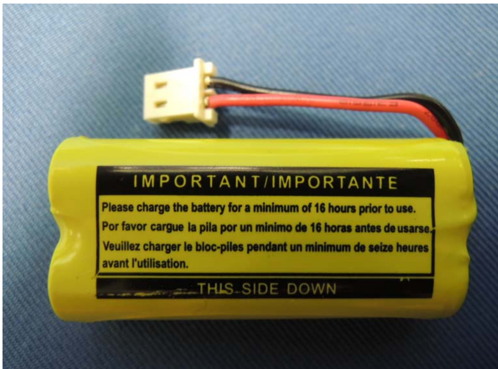
Figure 6 – 550mAh BYD battery back view
