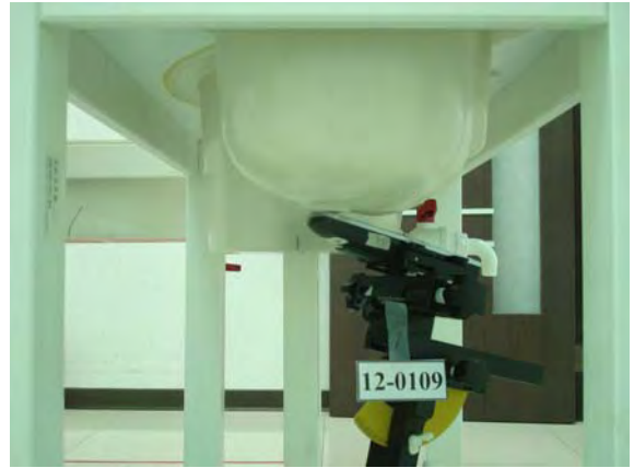
Figure 3. Right Head SAR Test Setup (Tilted)
