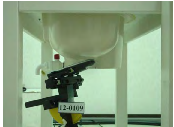
Figure 5. Left Head SAR Test Setup (Tilted)
