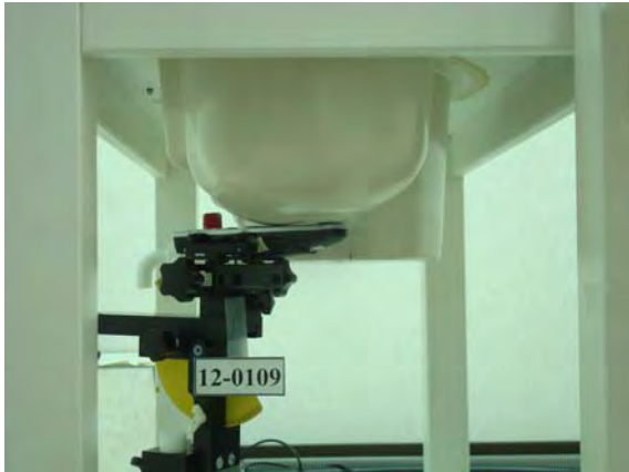
Figure 4. Left Head SAR Test Setup (Cheek)
