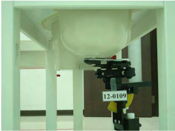
Figure 2. Right Head SAR Test Setup (Cheek)
