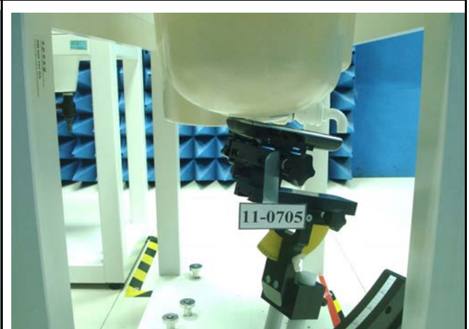
Figure 3. Right Head SAR Test Setup (Tilted)
