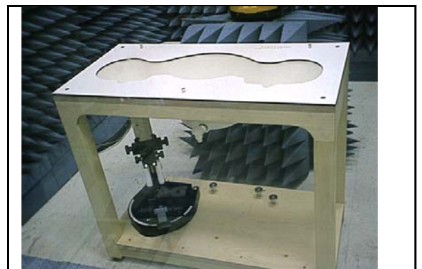
Figure 6. SAM Twin Phantom
