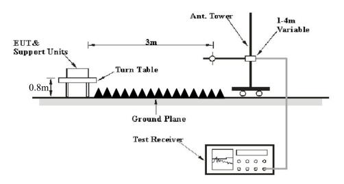
The radiated emission tests were performed in the 3 meters, using the setup accordance with the ANSI C63.10-2013. The specification used was the FCC 15.209 and FCC 15.319 (g) limits.
