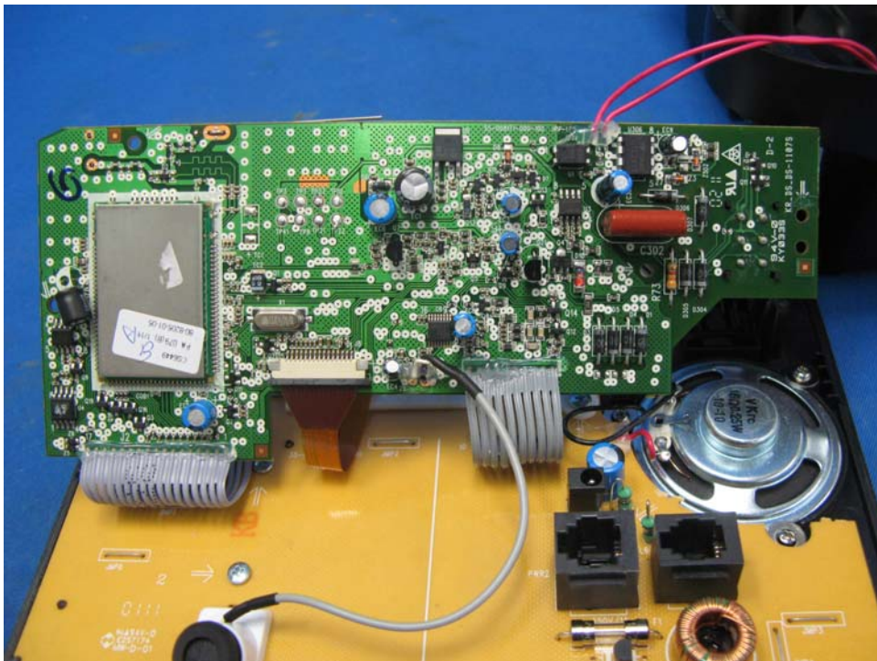
Base Unit Main PCB comp side
