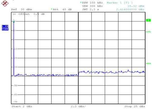
**Out Band Antenna Conducted Emission Plots**
