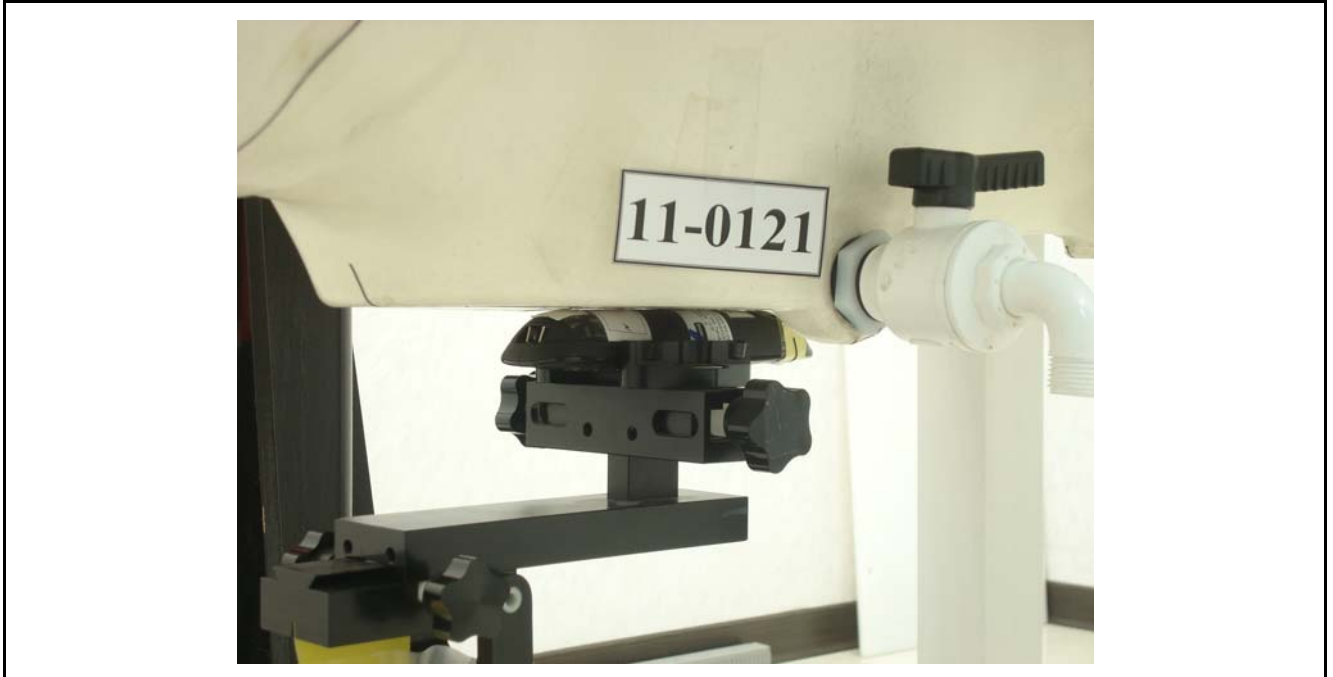
Figure 6. Body SAR Test Setup (Flat Section)
