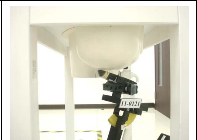
Figure 3. Right Head SAR Test Setup (Tilted)
