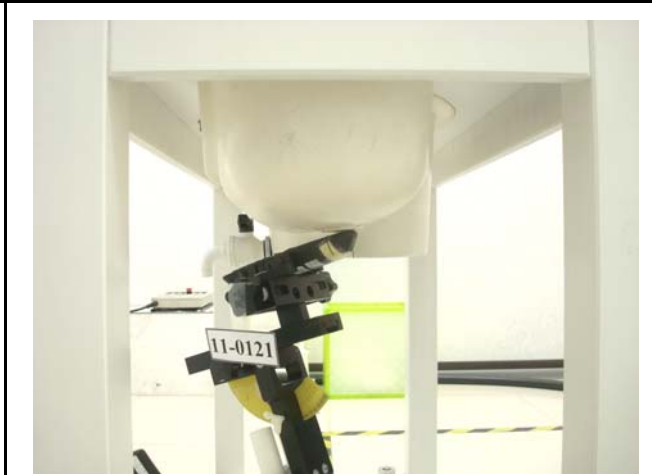
Figure 5. Left Head SAR Test Setup (Tilted)
