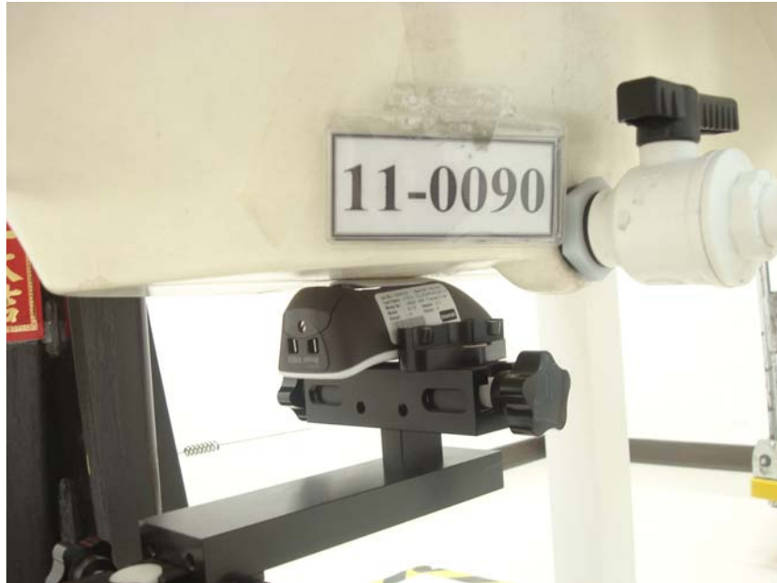
Figure 2. Body SAR Test Setup (Flat Section)
