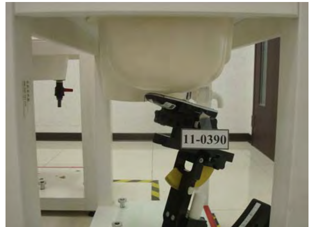
Figure 3. Right Head SAR Test Setup (Tilted)
