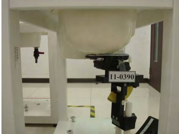
Figure 2. Right Head SAR Test Setup (Cheek)
