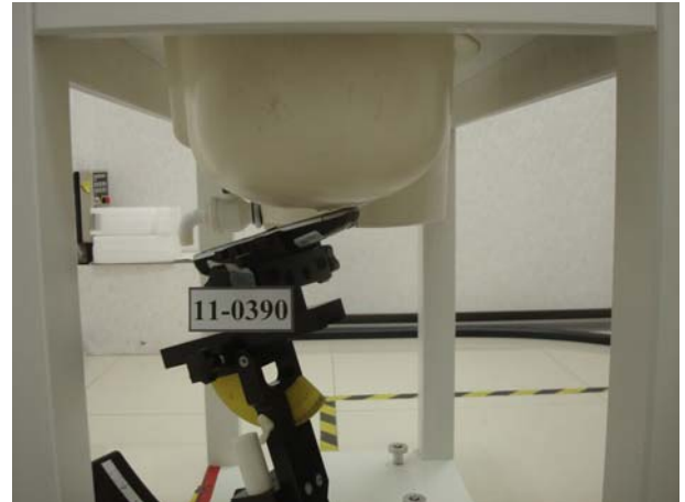
Figure 5. Left Head SAR Test Setup (Tilted)
