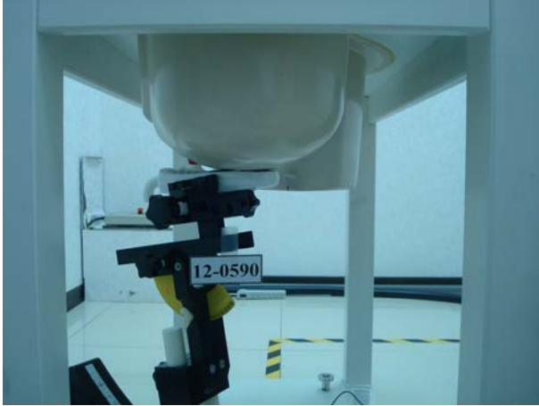
Figure 4. Left Head SAR Test Setup (Cheek)
