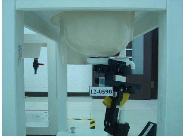
Figure 2. Right Head SAR Test Setup (Cheek)
