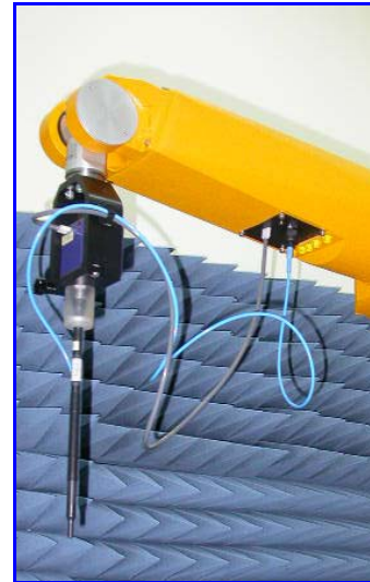
Figure 4. Probe setup on robot
