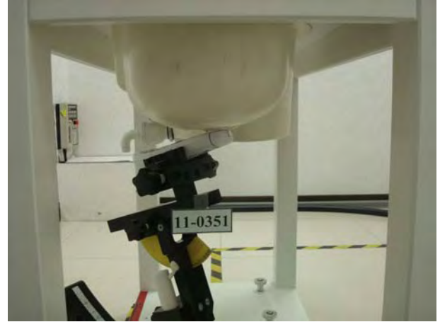
Figure 5. Left Head SAR Test Setup (Tilted)
