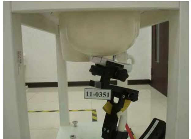
Figure 3. Right Head SAR Test Setup (Tilted)
