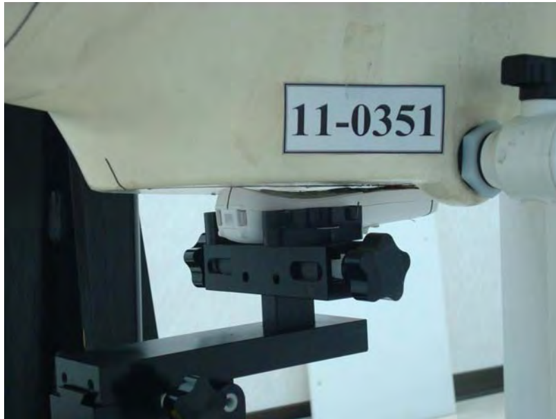
Figure 6. Body SAR Test Setup (Flat Section)
