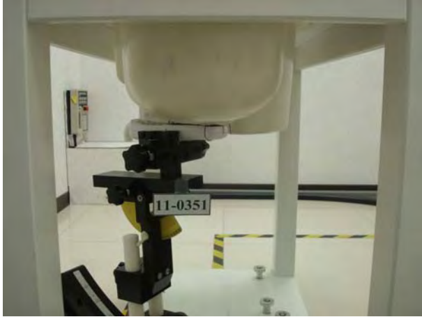
Figure 4. Left Head SAR Test Setup (Cheek)
