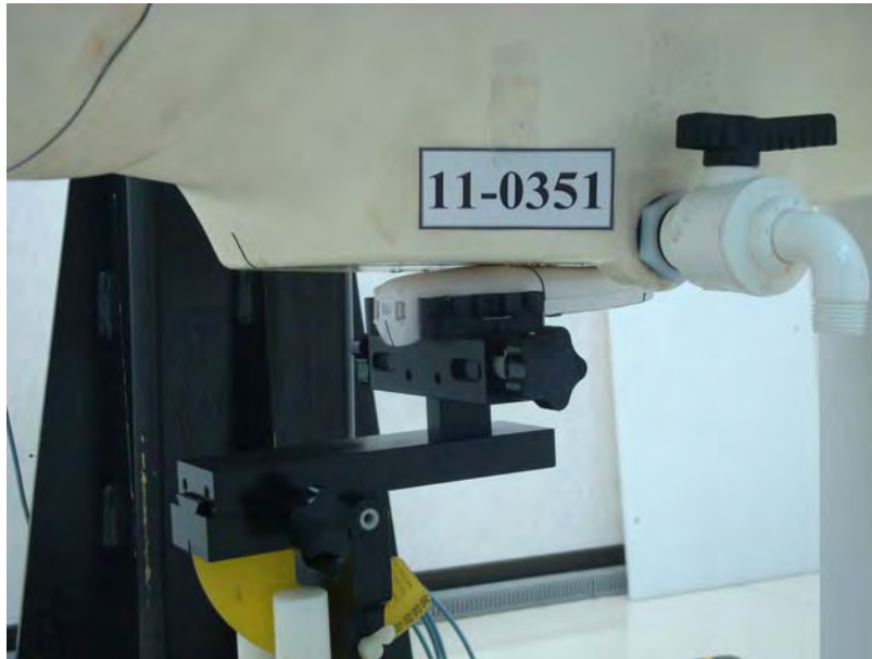
Figure 7. Body SAR Test Setup (Flat Section)
