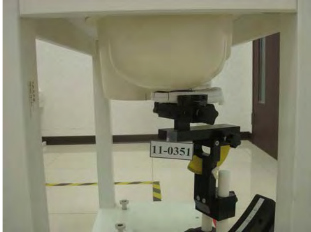
Figure 2. Right Head SAR Test Setup (Cheek)
