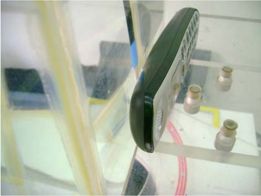
EUT rear to phantom, 0 mm separation – Zoom In
