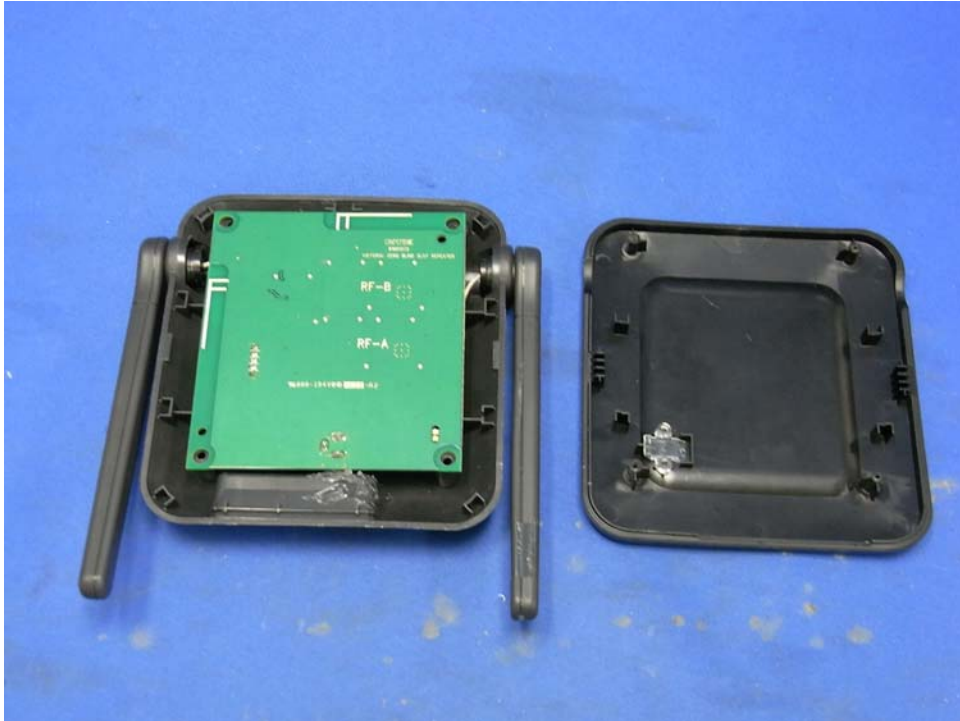
Repeater assembly (View 1)
