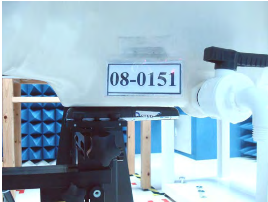
Figure 18. Body SAR Test Setup _ Back to Phantom 0mm separation
