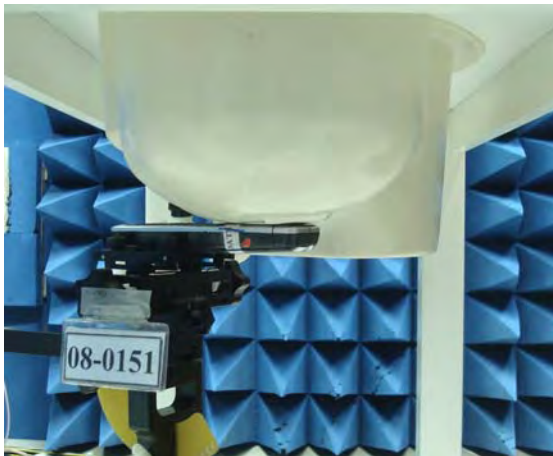
Figure 16. Left Head SAR Test Setup (Cheek)
