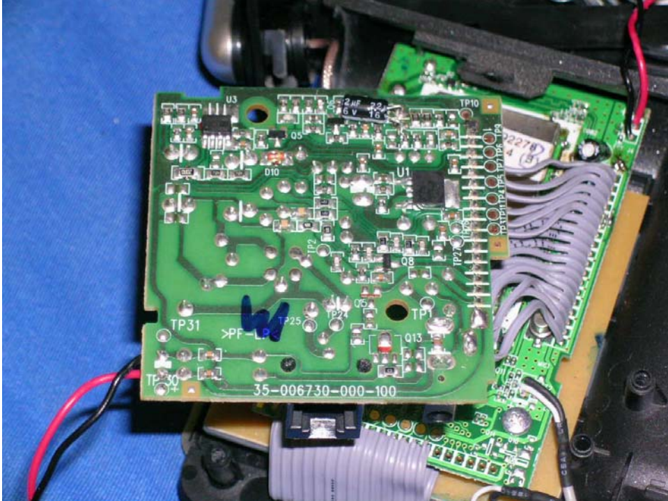
Base Unit Main PCB solder side
