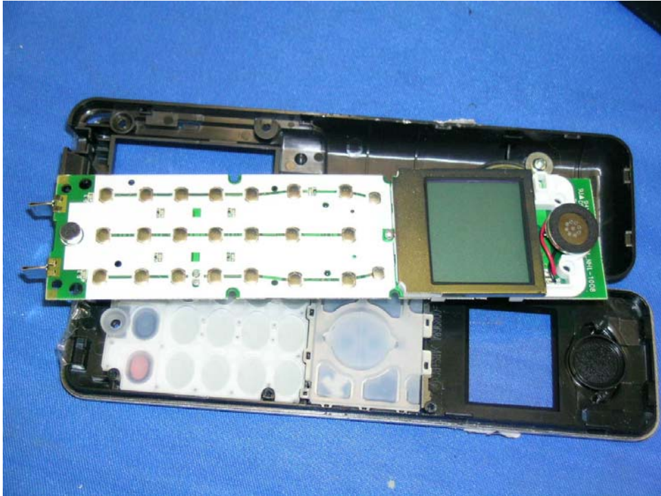
Handset Main PCB display side (View 1)
