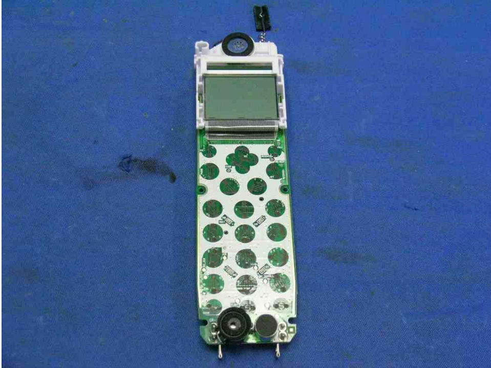
Handset Main PCB display side
