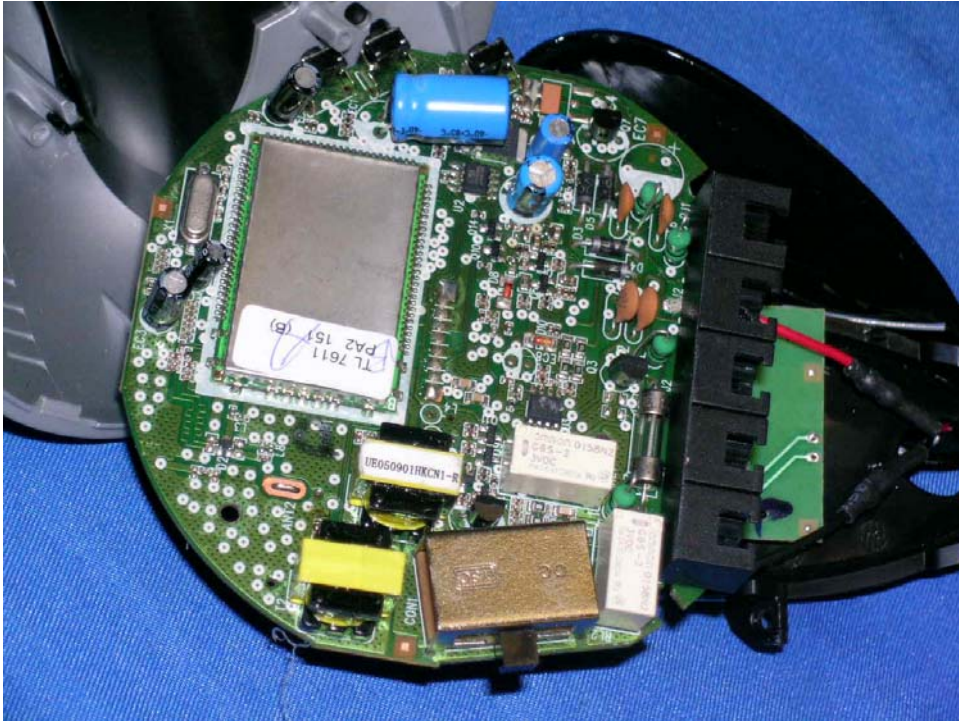
Base Unit Main PCB comp side
