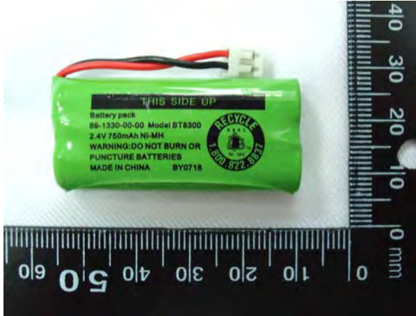
Figure 2. Battery (Ni-MH 2.4V , 750mAh)
