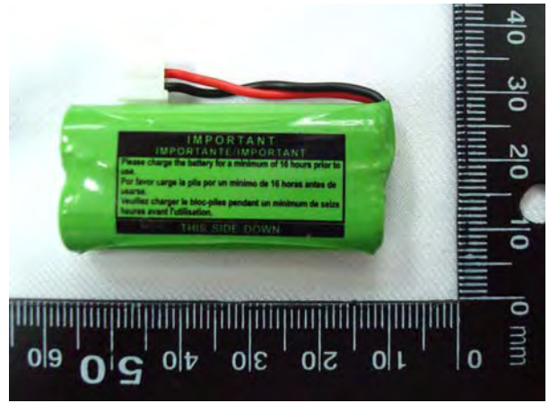
Figure 2. Battery (Ni-MH 2.4V , 750mAh)
