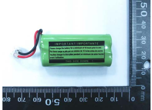
Figure 2. Battery (Ni-MH 2.4V , 500mAh)
