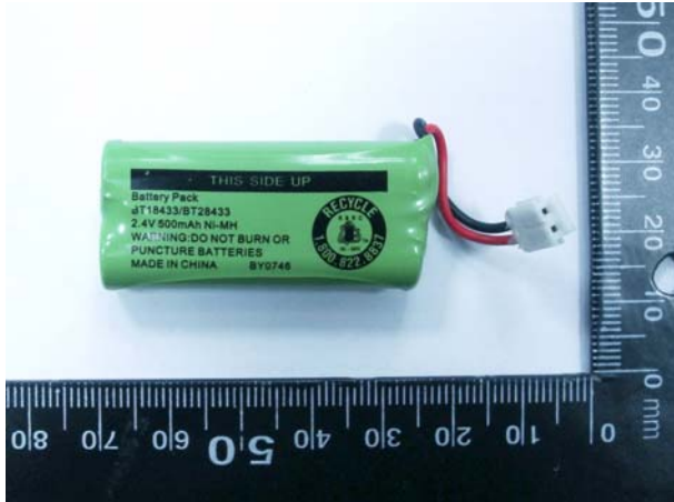
Figure 2. Battery (Ni-MH 2.4V , 500mAh)
