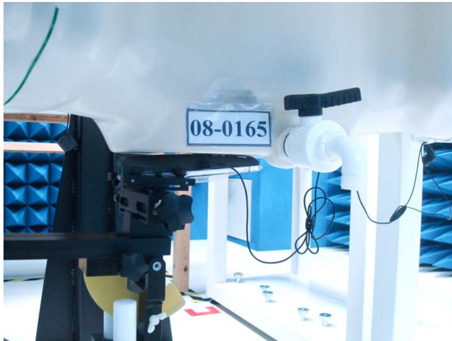
Figure 19. Body SAR Test Setup _ Back to Phantom 0mm separation
