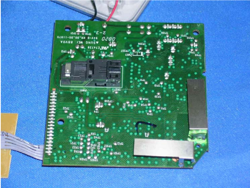
Base Unit Main PCB solder side
