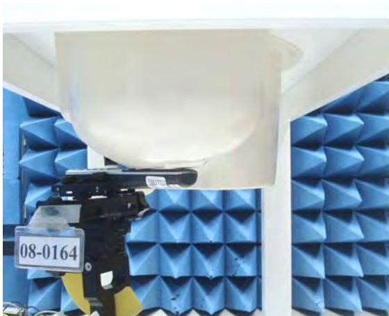
Figure 16. Left Head SAR Test Setup (Cheek)
