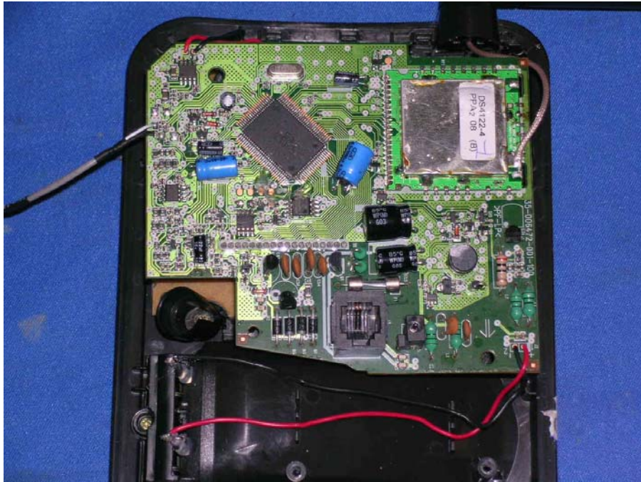
Base Unit Main PCB comp side
