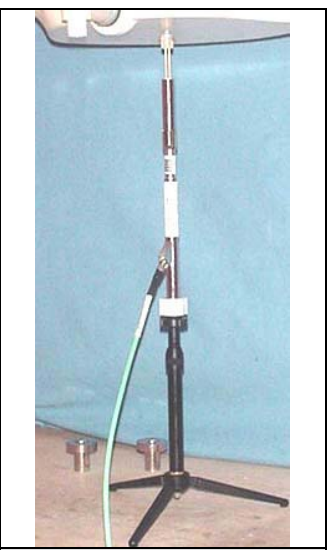
D5GHzV2 Dipole Setup
