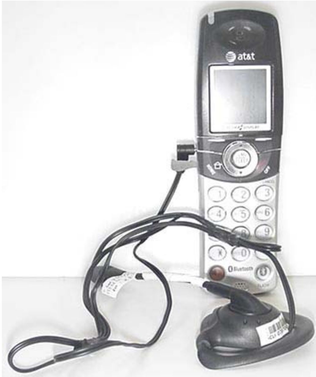
DUT with Generic Headset-Microphone Audio Accessory
