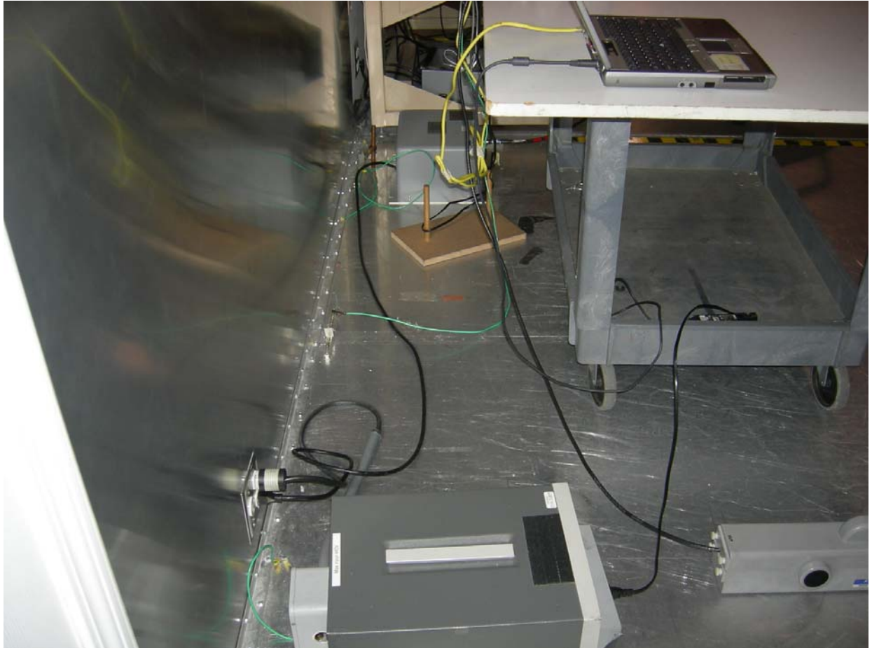
Figure 4: AC Power Line Conducted Emissions
