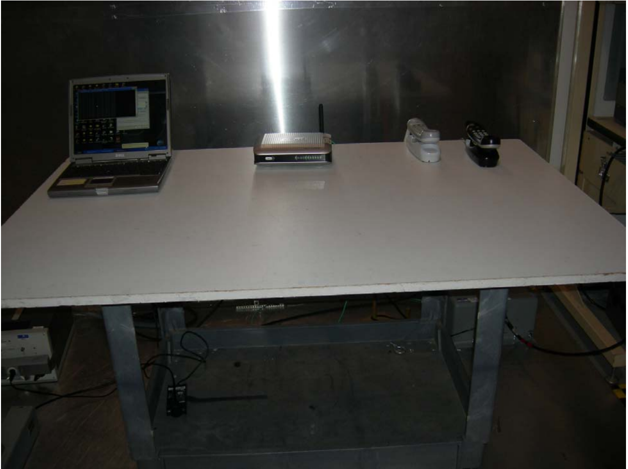
Figure 3: AC Power Line Conducted Emissions
