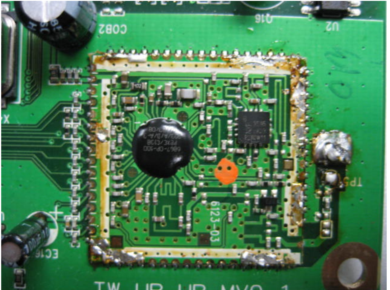
Figure 3: Close up of RF section without Shields
