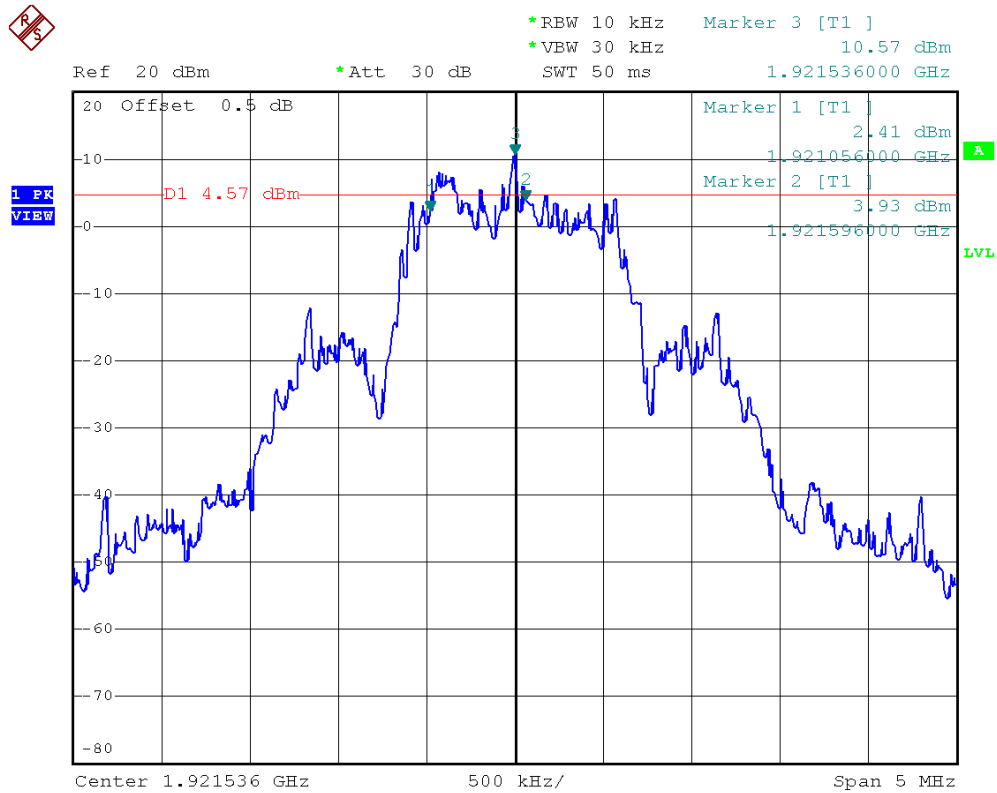
Plot 1H. Lowest Channel Test Frequency at -6dB points (Dummy Carrier)
