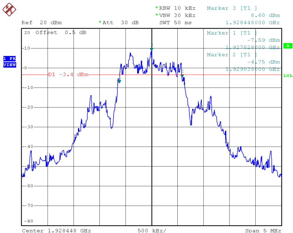
Plot 1L. Highest Channel Test Frequency at -12dB points (Dummy Carrier)
