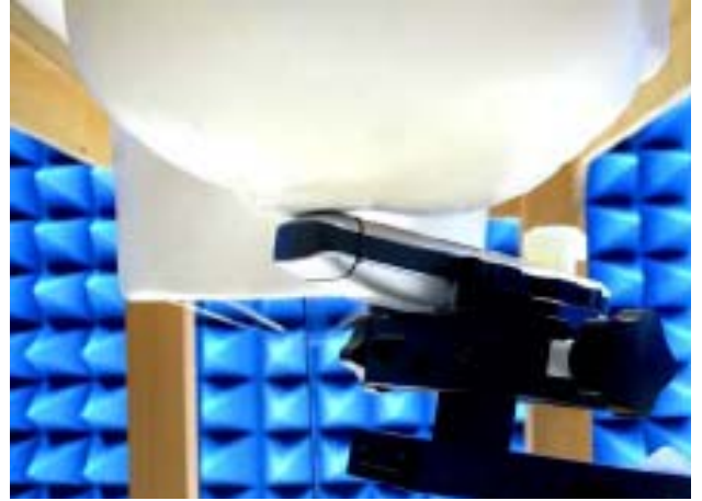
Figure 17. Right Head SAR Test Setup (Tilted)
