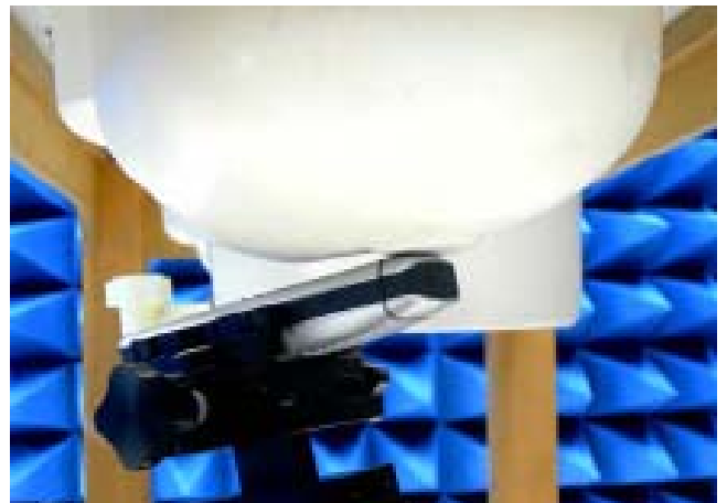
Figure 19. Left Head SAR Test Setup (Tilted)
