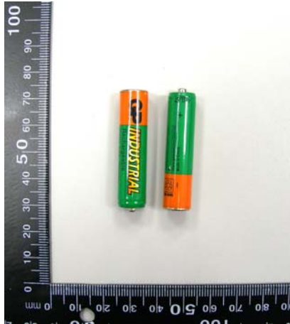
Figure 2. Battery (Ni-MH 1.2Vx2 , 750mAh)
