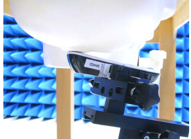
Figure 18. Right Head SAR Test Setup (Tilted)
