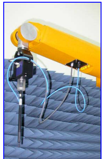
Figure 11. Probe setup on robot
