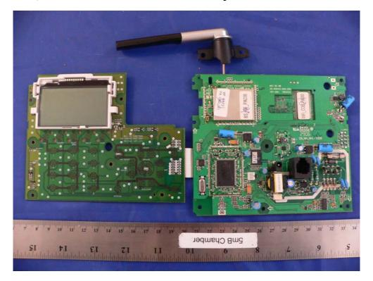
EUT – (WF6972) Base-set Main Boards with antenna Component View -2
