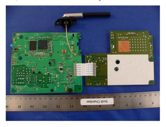
EUT – (WF6972) Base-set RF Board Detail View (RF Shielding Removed)
