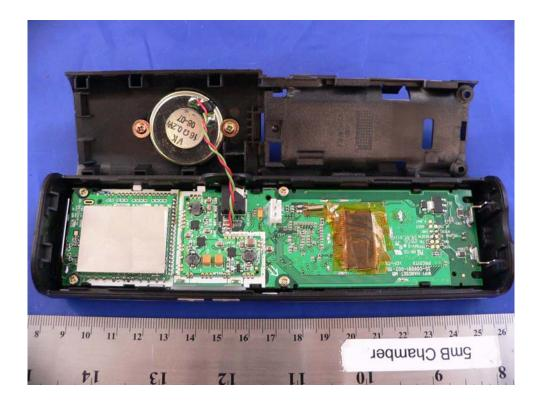
EUT - (WF6972 & WF6909) Hand-set Main Board Component View
