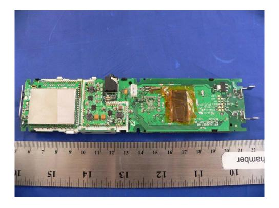
EUT – (WF6972 & WF6909) Hand-set RF Board Component Detail View (RF Shielding removed)
