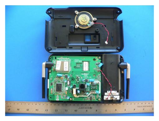
EUT – (WF6972) Base-set Main Boards with antenna Component View -1
