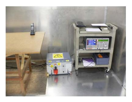
**AC Line Conducted Emission - Side View**
