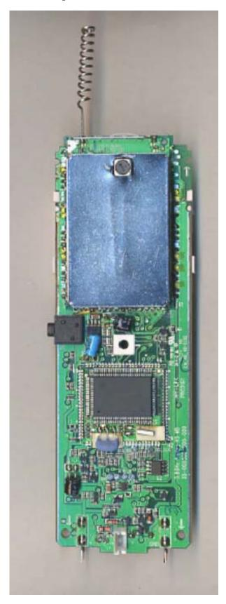
**EUT – Component Shielding Off View**
