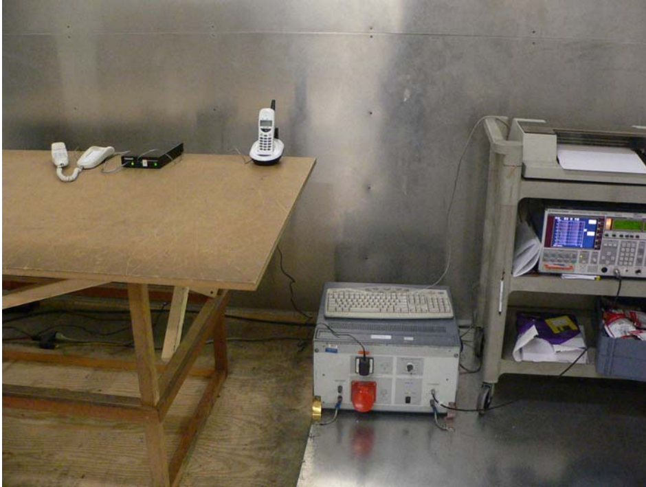
Conducted Emission - Front View
