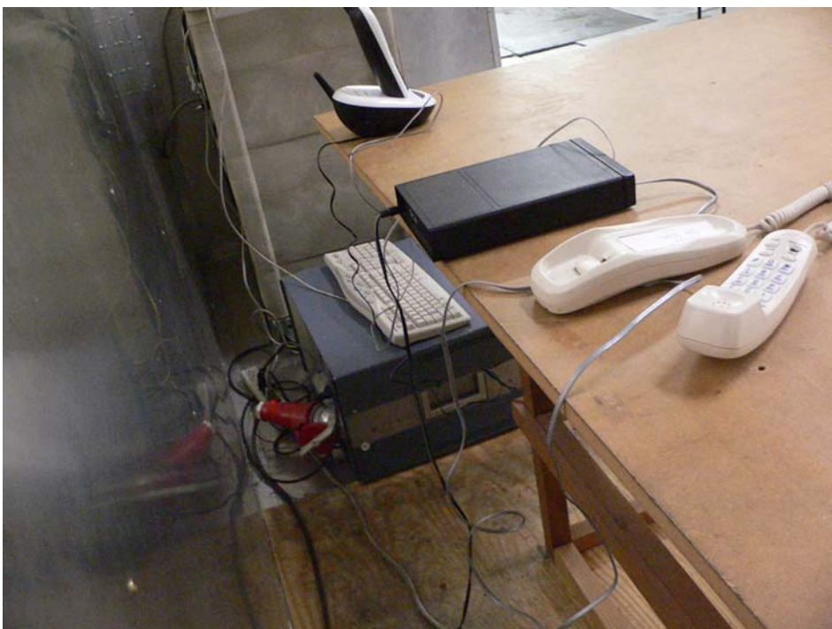
Conducted Emission - Side View
