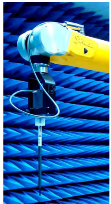
Figure 10. Probe setup on robot
