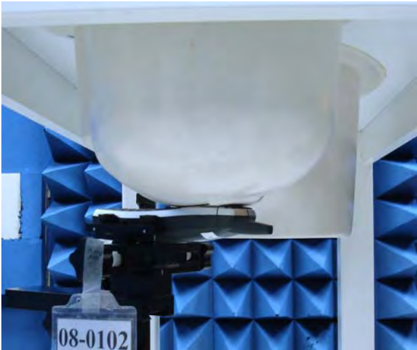
Figure 18. Left Head SAR Test Setup (Cheek)
