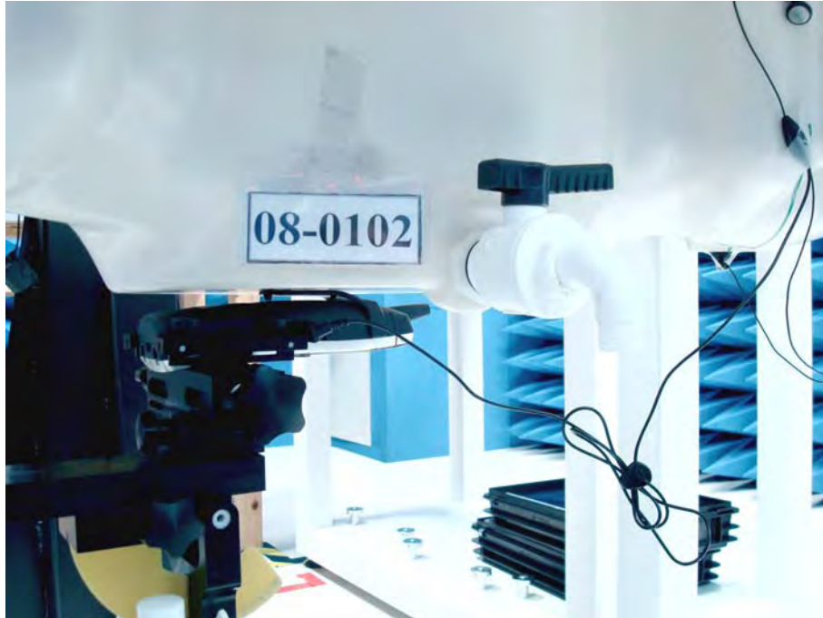
Figure 20. Body SAR Test Setup(Flat Section) with belt clip and Headset
