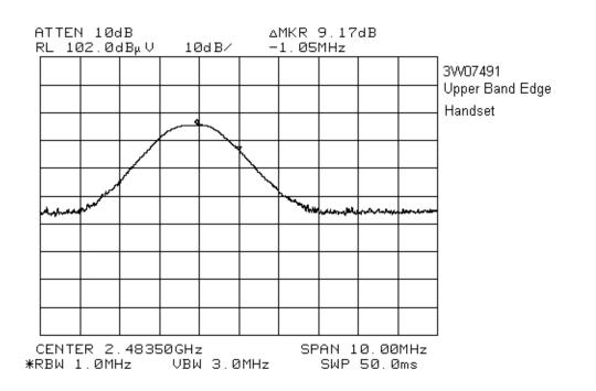
Peak Level Band Edge: 79.8dBuv + 34.8dB - 9.2dB = 105.4dBuV/m@3m Peak Band Edge Level (Marker Delta): 105.4dBuv/m - 46.8dB = 58.6dBuV/m@3m Average: 58.6dBuV/m - 20.0 = 38.6dBuV/m@3m
