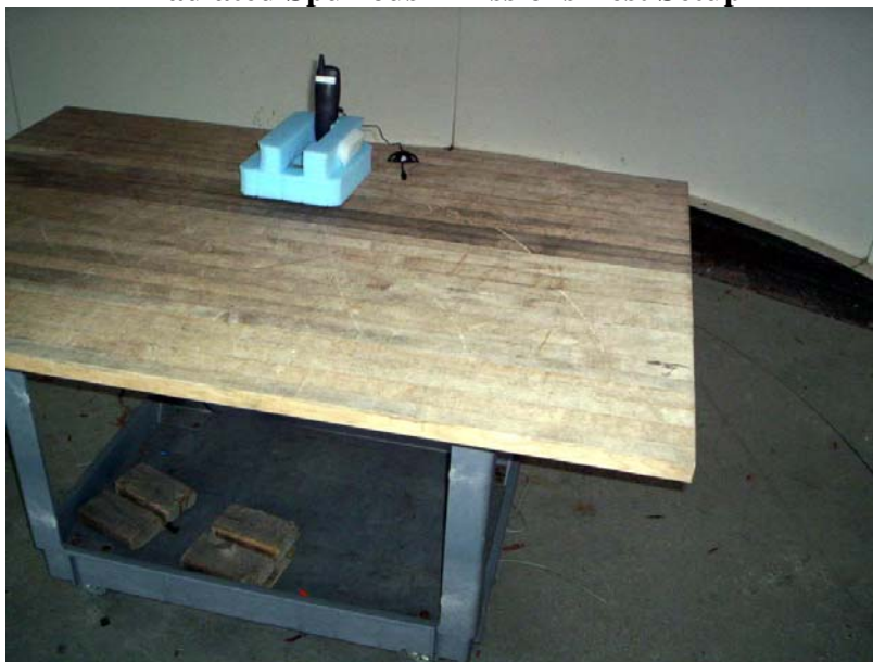
Radiated Spurious Emissions Test Setup
