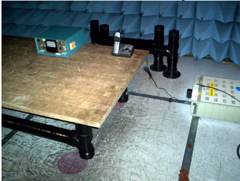
Conducted Emissions Test Setup:
