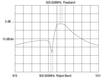
Figure 3 High band ceramic filter response
