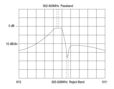
Figure 2 Low band Ceramic filer response
