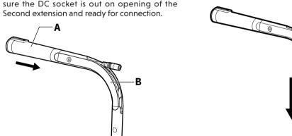
3. Let the cable jack of the Extension cable pass through from the back of the Mounting cover (D), to the opening of the Second extension (B).
