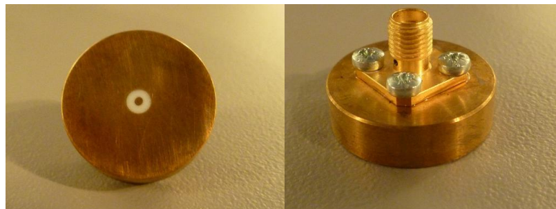
Figure 1 – MVG LIMESAR Dielectric Probe
