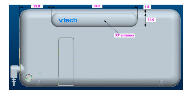
Figure 1 Physical dimension (mm)
