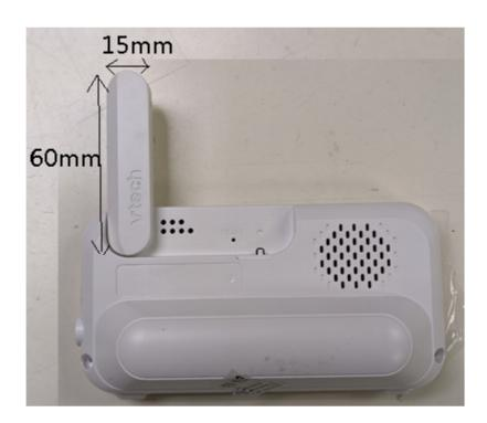
Figure 1 Physical dimension (mm)
