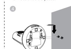
Align the wall mount holes on the baby unit with the screws on the wall. Slide the baby unit down until it locks into place.
