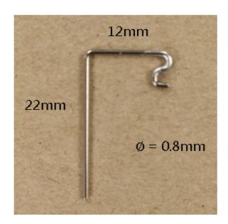
Figure 1 Physical dimension (mm)
