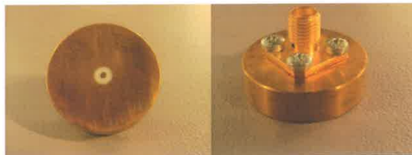
Figure 1 – MVG LIMESAR Dielectric Probe
