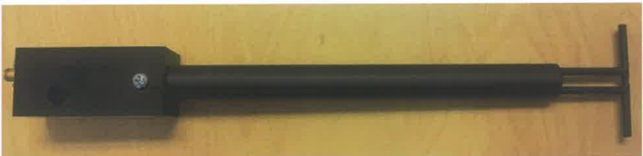
Figure 1 – MVG COMOSAR Validation Dipole
