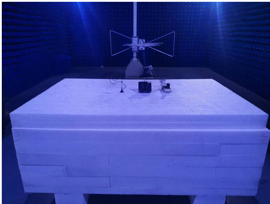
Photo of Radiated Emission Measurement (Above 1G)
