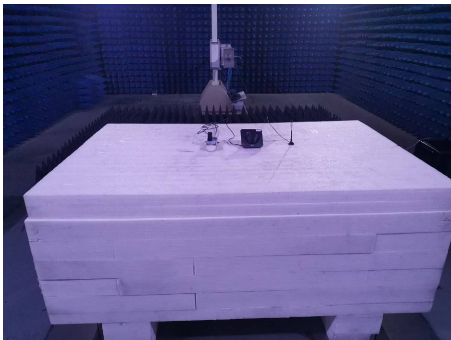
Photo of Radiated Emission Measurement (Above 1G)
