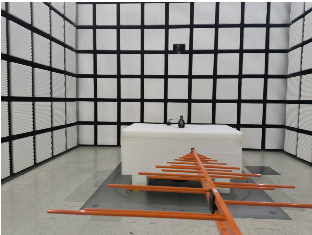
Radiated Emission Below 1GHz View
