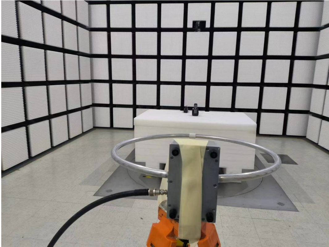
Radiated Emission Below 1GHz View
