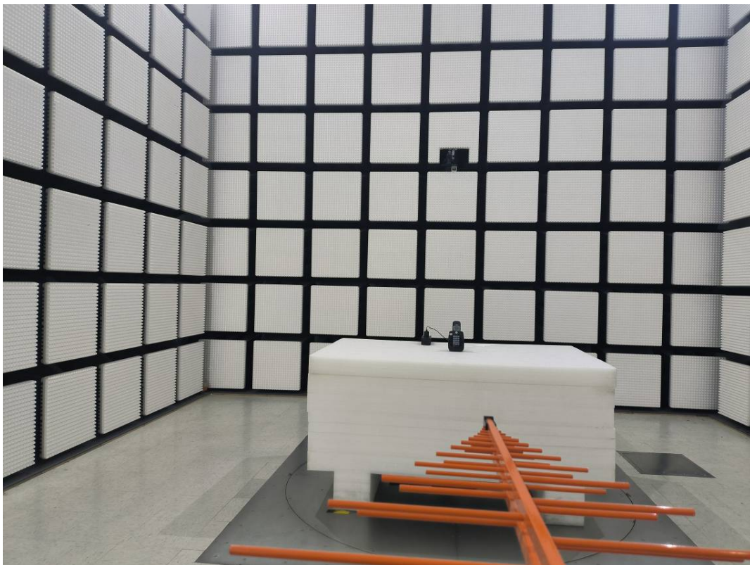
Radiated Emission Below 1GHz View
