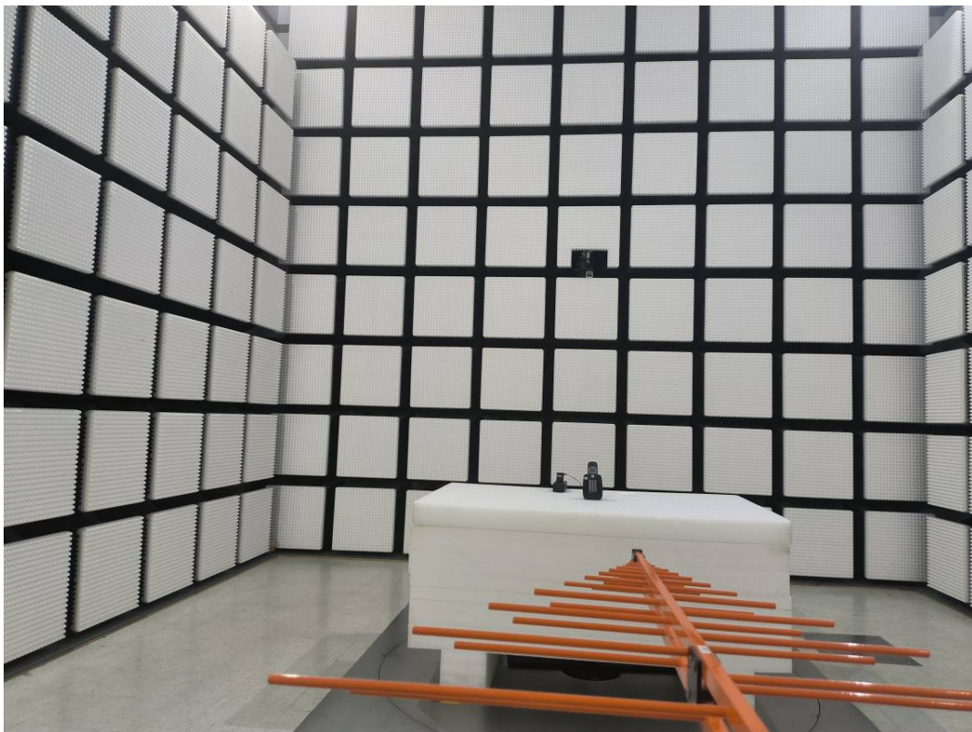
Radiated Emission Below 1GHz View
