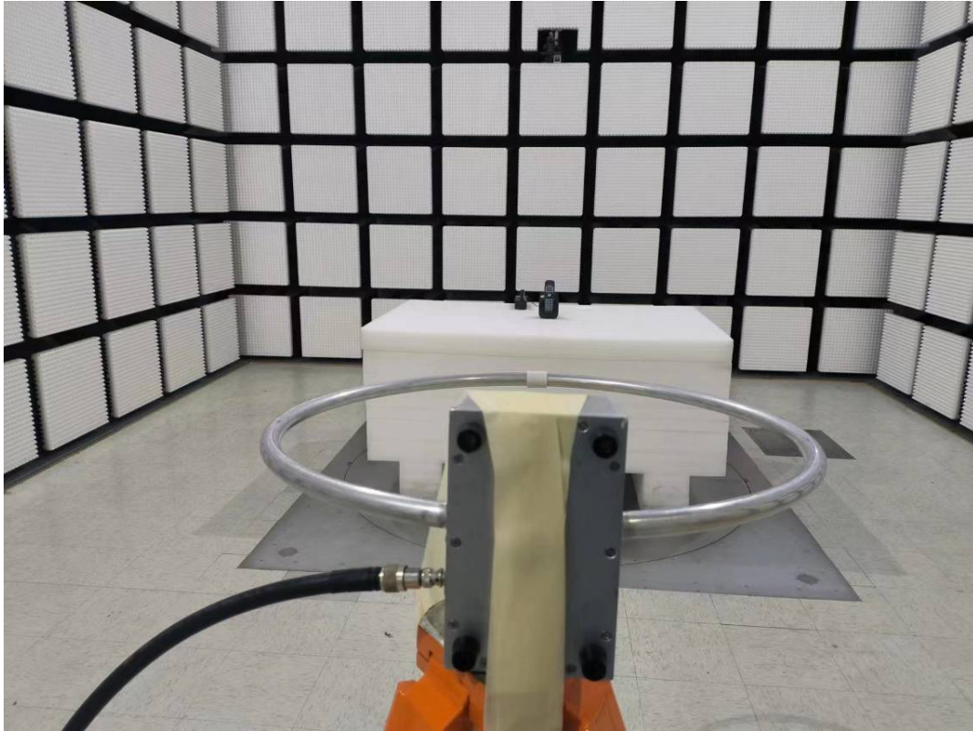
Radiated Emission Below 1GHz View
