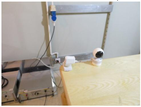
Radiated Emissions (30MHz-1GHz) Test Setup
