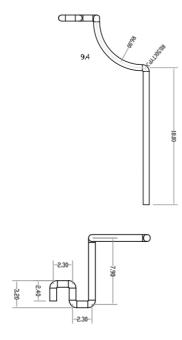
Figure 1 Physical dimension (mm)
