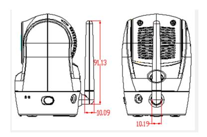
Figure 1 Physical dimension (mm)
